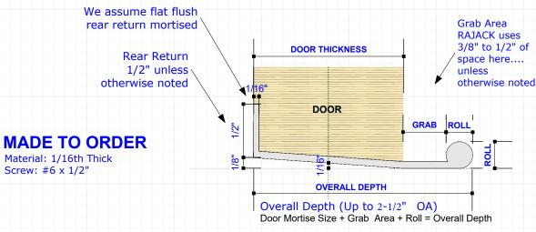
Note: screw holes can be placed on rear return only. Upon request. This is only recommedned on pulls 4"L or less.
